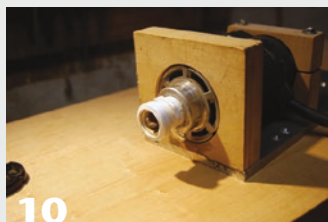
10 Router mounted in carriage with PVC depth gauge collar.
