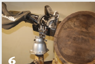
6 The biscuit joiner mounted on the gimbal, mounted in the lathe banjo, ready to cut slots across a crack in a bowl wall. Note: cutter blade extended for illustration purposes only.
