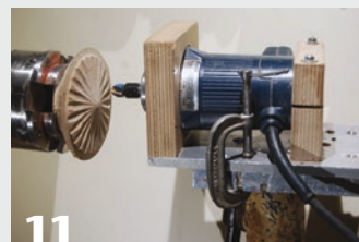
11 Platform mounted in banjo with router carriage clamped to it. The router is aligned with rotation axis and ready to cut a rosette.
