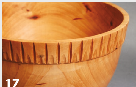
17 Two passes using different router bits.
