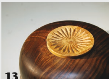
13 A convex and concave rosette ( Photos 12 and 13 , respectively), both routed at the lathe.
