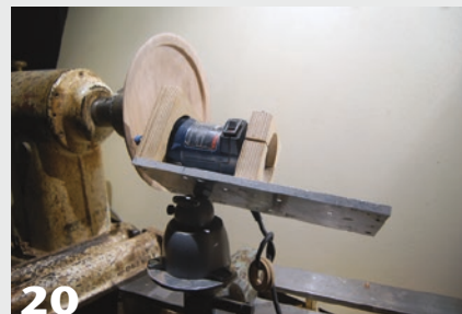
A router carriage with gimbal post allows for router rotation and an "arc" cutting pattern.
