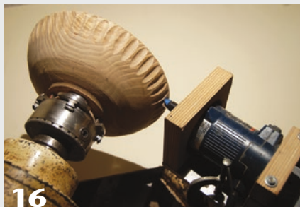
16 With the router mounted perpendicular to the turning axis, many possibilities exist for rim treatments.
