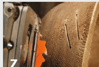
6 The biscuit joiner mounted on the gimbal, mounted in the lathe banjo, ready to cut slots across a crack in a bowl wall. Note: cutter blade extended for illustration purposes only.
